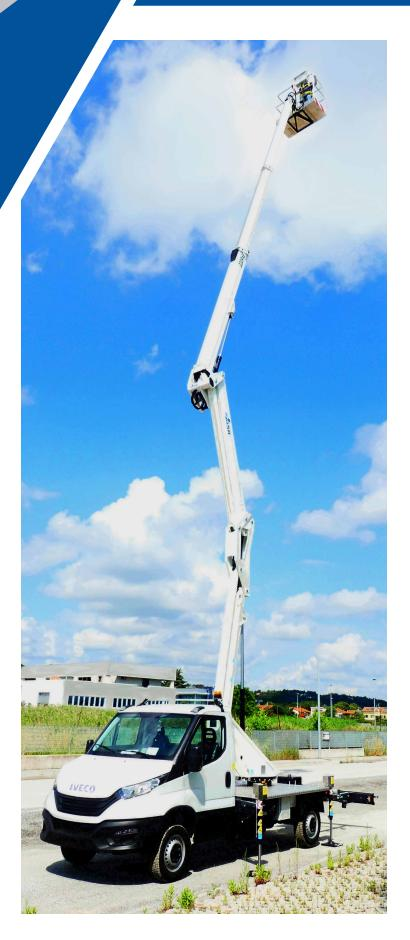
The new B220PXE platform integrates the double "up-and-over" articulation with an innovative telescopic boom and end mounted basket.
